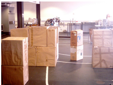
Figure 7: Experimental setup with two narrow passages built with paper boxes with one of them blocked ahead.
