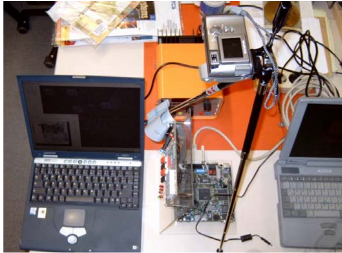
Fig. 6. Remote FPGA server (right), FPGA board (middle) and user client (left).
