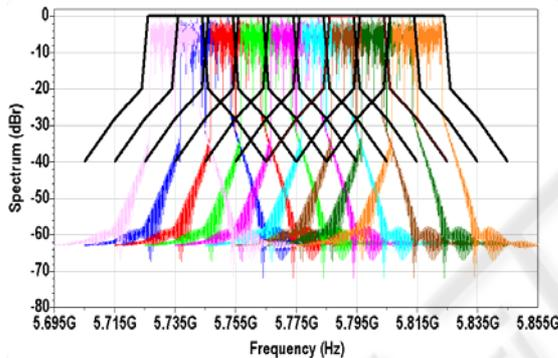
Figure 1: Transmit RF Spectrum
