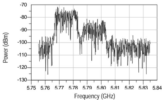
Figure 3: Adjacent Channel Rejection
