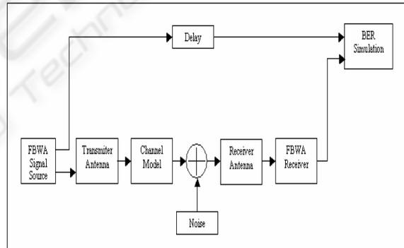
Figure 9: Block Diagram for Simulation
