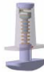
Figure 9: Design of the pseudo haptic input device prototype.
