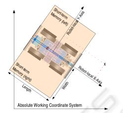
Figure 5: Schema of how to determine whether an obstacle representative resides in the blind region of the vehicle.
