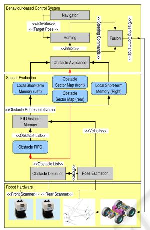
Figure 3: Top-level concept of RAVON's Obstacle Avoidance Facility.
