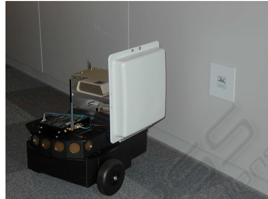
Figure 1: RFID tag pasted on a wall (white panel on right) and the antenna of a RFID tag sensor mounted on a mobile robot.
