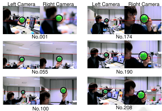
Figure 12: Several frames in the sequence for tracking a target in the zoom-focus control experiment.
