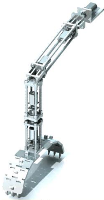
Figure 2: Kinematic configuration of a leg.
