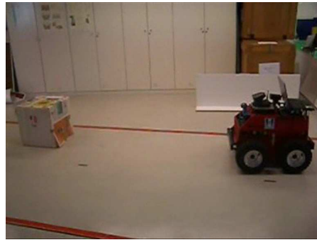
Figure 2: The HANS vehicle (ATRV robot) in the test environment; note the obstacle ahead in the "road".
