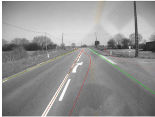
Figure 2: Detected lane-markings (in green) and uncertainty about curve position (in red).
