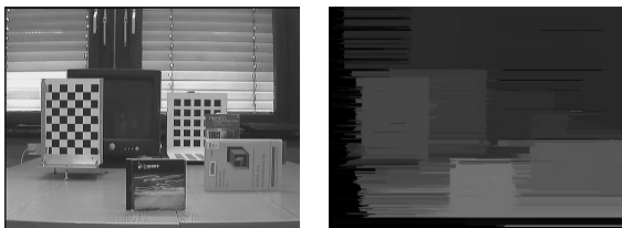
Figure 7: Left image of the experimental setup (left) and associated disparity map to determine optimal baseline offset.
