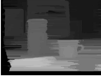
Figure 5: 2.5 dimensional depth map. The darker a pixel the farer away from camera.
