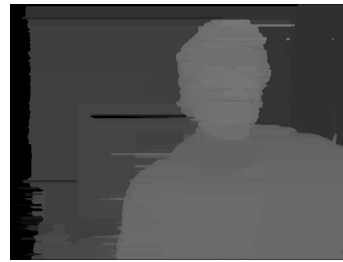
Figure 9: 2.5 dimensional depth map of a face. The darker a pixel the farther away from camera.
