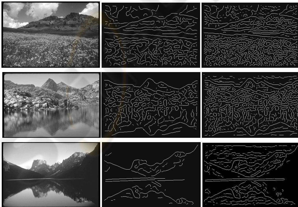
Figure 1: Three sample images in our image database and the corresponding two-scale canny edge images.
