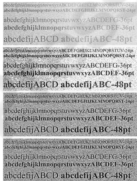
Figure 9: From top to bottom: Results of the OFF ganglion cells ( G ), final result of the proposed method ( B ), Sauvola’s and Niblack’s results for the 90% SH image with 0.2 noise variance.
