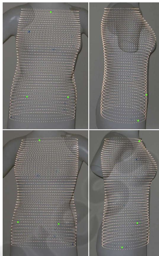
Figure 4: The 4 images of a dummy torso with the anatomical landmarks used to compute the initial registration (green dots). Projection of the initial model is superimposed.
