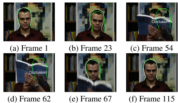
Figure 3: Selection of result frames to indicate the performance of the AC-AAM tracker. The green and white shapes are the output of active contours and AC-AAM respectively. Note that the AC-AAM provides no AAM when the object undergoes occlusion in (c) and (d).
