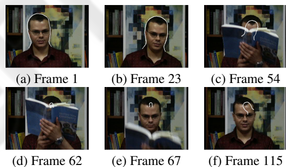
Figure 1: Selection of result frames illustrating the performance of the deterministic AAM tracker. In (c) and (d) the tracker loses its target due to the presence of occlusion and is not able to recover the target as shown in (e) and (f).
