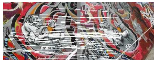
Figure 3: Example of matching results with the Graf sequence: 71 correct matches are found between the first and fourth frames.
