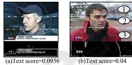
Figure 3: Shot text scoring. The text score of a frame containing text (a) is greater than a frame not containing text (b).
