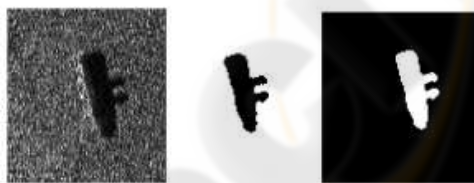
Figure 2: A real Sonar image involving sea floor and a man-made object (trolley) (a:left image). Extracted cluster "Shadow" (b: middle image). Complement of the cluster "Shadow" (c: right image).
