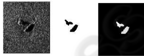
Figure 10: A real Sonar image involving an object and a rock shadows (a:left image). Extracted cluster "Shadow" (b: middle image). Complement of the cluster "Shadow" (c: right image).
