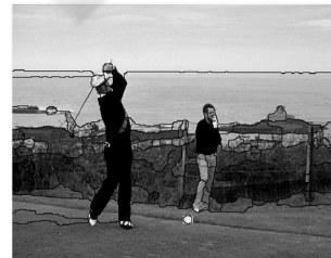
Figure 9: Segmentation performed by applying the watershed transform.
