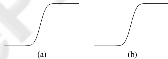
Figure 4: A smoothed step like boundary response is shown in (a) and the result post median filtering in (b).
