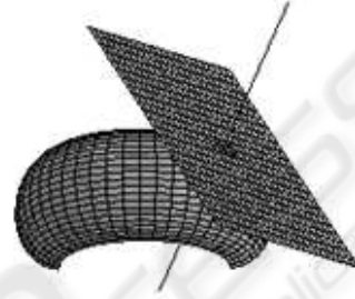
Figure 1: A surface with its tangent plane and normal vectorial space at a point.
