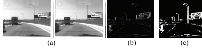
Fig. 2. Movement detection based on image difference. (a) Image sequence (b) Absolute value of image differences (c) thresholding of the previous images.
