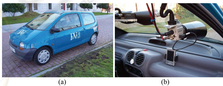
Fig. 9. IVVI Vehicle. (a) Experimental Vehicle (b) stereo and color camera.
