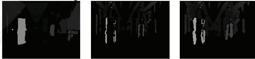
Fig. 6. Disparity Map Results: On the left side our method, on the center side the SSD, and on the right side the SSD multi-scale.
