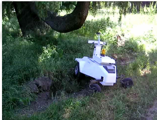
Fig. 6. Outdoor robot in typical terrain. Robot is part of a DARPA project, Learning Applied to Ground Robotics. Two stereo systems are on the upper crossbar.
