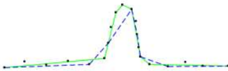
Figure 5: SimpliPoly (solid line) vs. Douglas-Peucker (dashed line): the original polyline (not shown) has 20 vertices (shown), while both simplifications have 8 vertices each, a reduction of 60%.
