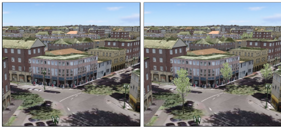
(a) trees projected on the ground (b) 3D model rendered on top the projected trees
