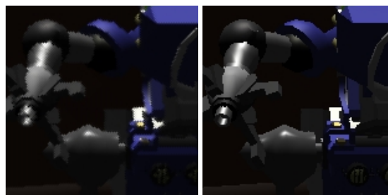
Figure 4: Interleaved rendering (left) leads to higher frame rates than normal rendering (right), but also to a blurred image (part of the BART robots scene (Lext et al., 2000)).
