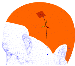
Figure 2: A key strand defining a wisp for a group of four triangles on the scalp. The dark area on the scalp defines the selected triangles. The blue square points are the control points on the key strand.
