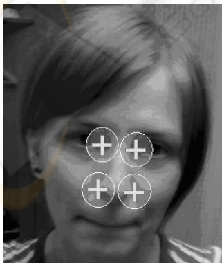
Figure 6: Search areas for tracking of two nose and two eyes inner corners.
