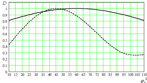
Figure 4: Application of the proposed method for reduction of direction finding systematic errors and increase of azimuth resolution on a mobile carrier (the full line shows the array pattern as in Figure 3 and the dash line shows the array pattern for the array with the triple diameter).
