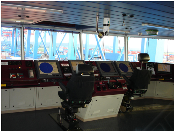
Figure 1: Bridge with high integration level.
