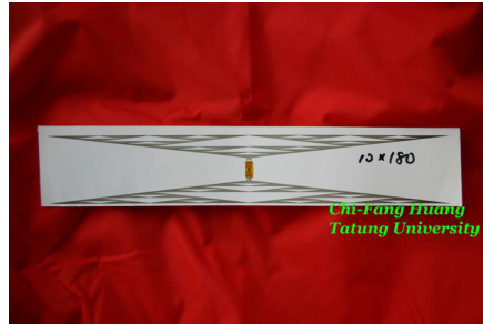
Fig. 8. A single RFID tag of UHF band made by offset printing technology.
