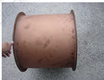
Fig. 3. Metal cylindrical cavity for measuring the ink’s conductivity.
