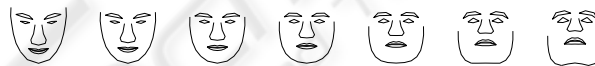
Fig. 3. Effect of changing the value b_1 on the reconstructed shapes. \phi_1 controls the up-down rotation of the face.
