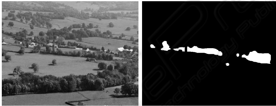
Fig. 2. A test image and its ground truth of the test image: white for buildings, black for vegetation.
