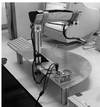
Figure 1: Device for arm support and joint angle monitoring.
