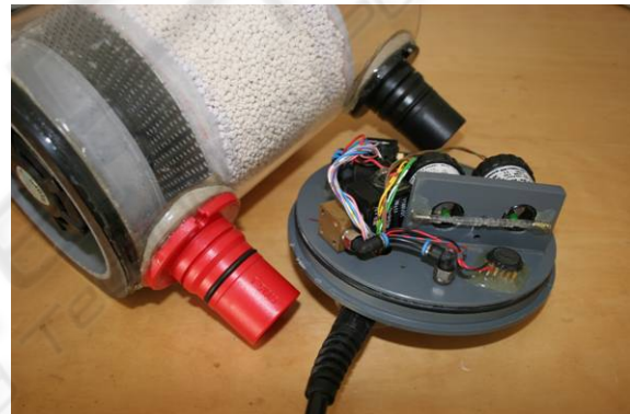
Figure 6: Scrubber and scrubber head with solenoids, pressure sensors and two pO 2 sensors (Analytical Industries, PSR 11-39-MD2).
