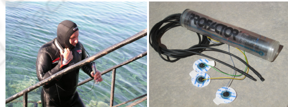
Figure 12 A,B: Francesco Colletta after 32h underwater and our especially for this dive adapted ECG measurement device (at the end of each of the two black cables one temperature sensor is encapsulated in epoxy resin).
