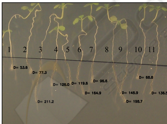
Figure 3: Image of growing roots with the software output overlaid. The root numbers refer to the results in Table 1.
