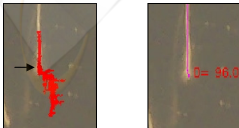
Figure 7: Left: A particle filter tracker will always try and hunt a target even if one does not exist, as the spread of particles past the root tip (indicated by arrow) shows. Right: An example result of the same root image with the new root termination criteria.
