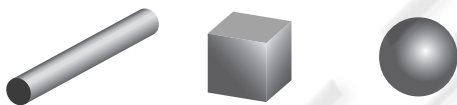
Figure 1: Long cylinder, cube and sphere of same volume ( V = 1000 ) have different surface ( S_{\text{cylinder}} = 694 (for this arbitrary proportion), S_{\text{cube}} = 600 , S_{\text{sphere}} = 484 ).
