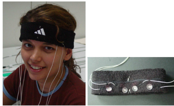
Figure 1: Headband, build-in electrodes at fp1, fp2, f7, f8.
