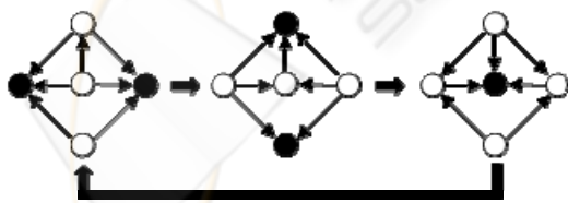
Figure 1: An example of the SER graph dynamics. Black nodes represent operating processes; white nodes represent idle processes.
