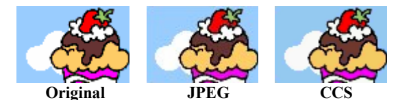
Figure 5: A detail of the "Benjerry" image compressed with the proposed pipeline (CCS) and with JPEG codec. The above detail shows the absence of artefacts (ringing) typically showed by JPEG engine.
