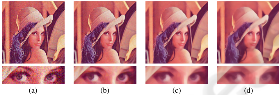
Figure 2: Anisotropic scale space for the Lena Image with 20% uncorrelated noise for each pixel in the input image: (a) Input image, (b) c=3 , (c) c=20 and (d) c=250 .
