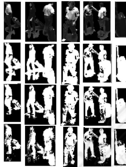
Figure 1: Captured images of different instances of single person , group of people , and luggage , with their associated blob and the blob after removing shadows in gray levels and RGB space.
