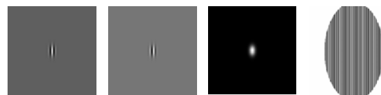
Figure 8: Real part, imaginary part, magnitude and phase of Gabor filter in the spatial domain. F=0.09375 ; \theta=0^\circ ; \sigma_x=6 ; \sigma_y=10 .
