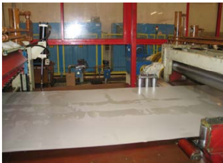
Figure 3: Coil slitting line (images courtesy of GONVARRI Group).
