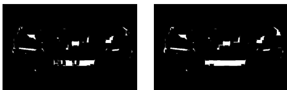
Figure 3: Left: Image after dilation/erosion with a window 15 pixels width. Right: Image after dilation/erosion with a window 20 pixels width.
