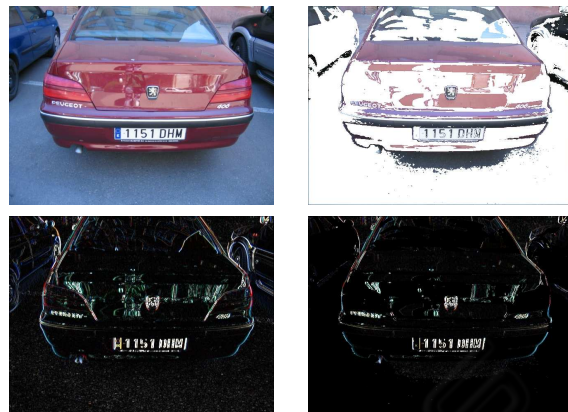
Figure 1: Top left: Original RGB image. Bottom left: After applying traditional Sobel filter. Top right: the image without the low saturation areas. Bottom right: After applying the conditional Sobel filter.
