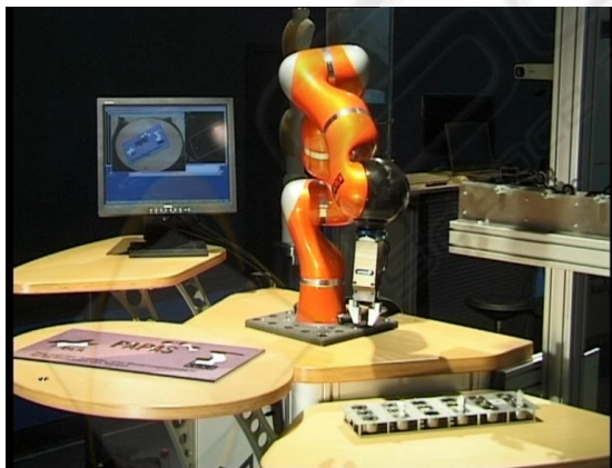
Figure 5: A light-weight robot arm as an assistant for human-like working in industrial environments the PAPAS experimental setup is designed to demonstrate a typical example of an industrial manufacturing process.
