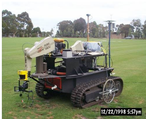
Figure 4: Autonomous Rough Terrain Tracked Robotic Vehicle.
