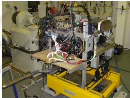
Fig. 1. View of engine test-bed and dynamometer.
