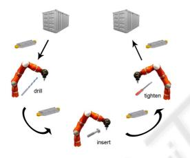
Figure 3: The adaptive production cell.
