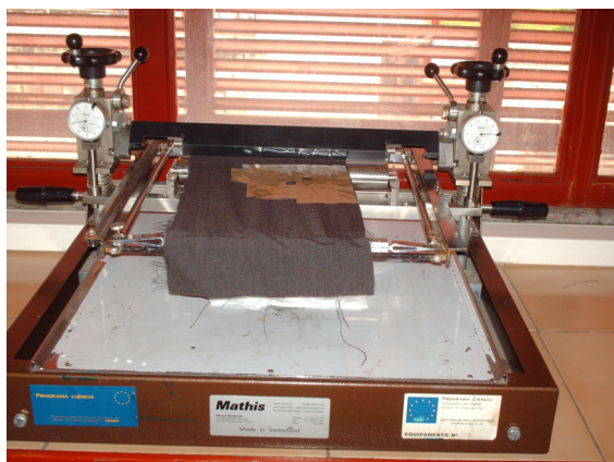
Figure 4: Electrode coating device.
