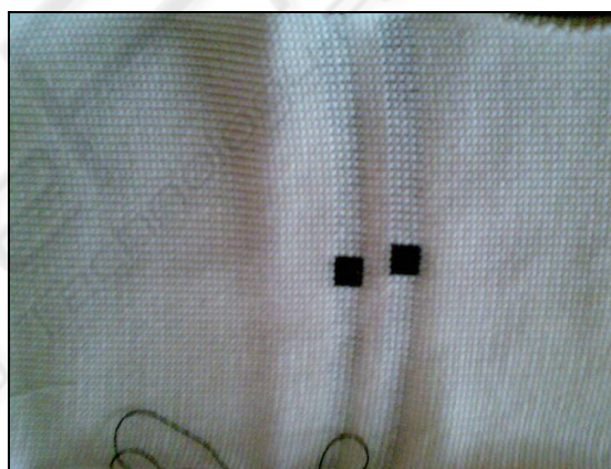
Figure 6: Knit right face with electrodes.
